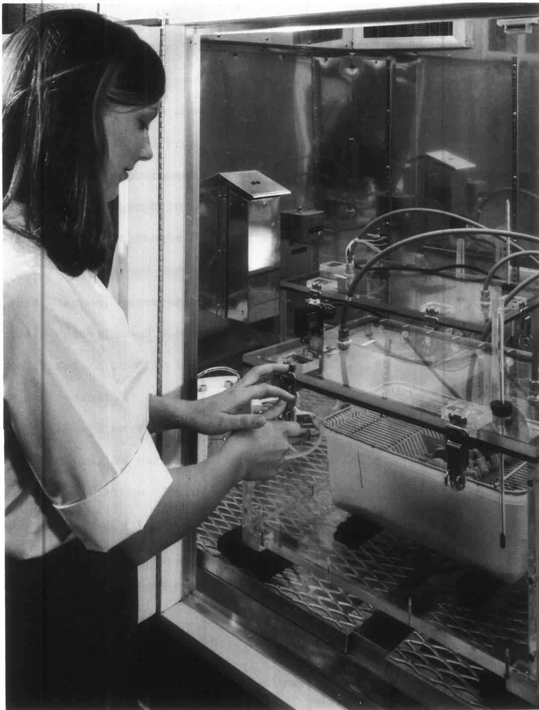
Figure 9. Specially constructed respiration chambers for holding rodents and cages in environment chamber during CO 2 measurements.
