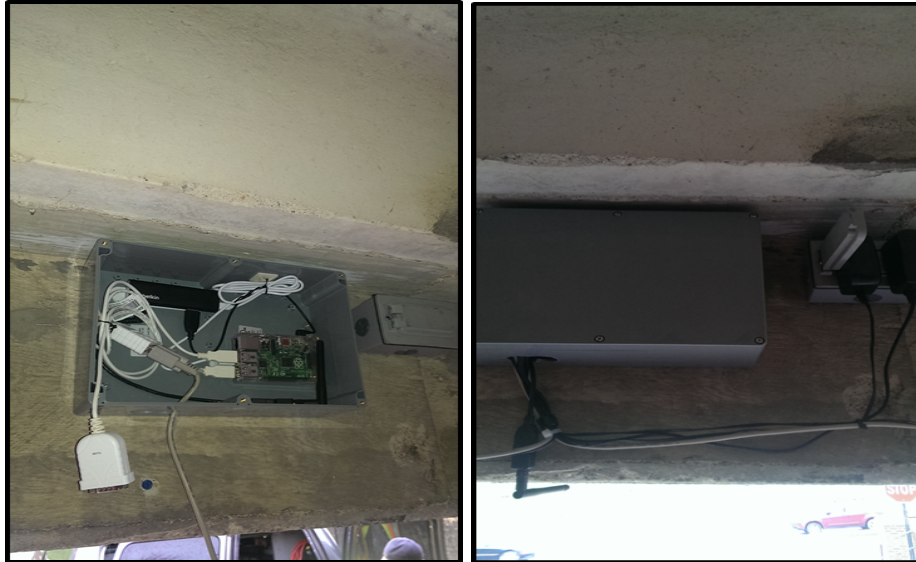
Figure 8. Main box holding the Raspberry Pi, Wi-Fi Antenna, USB Hub, and cable slack. Stowed in the upper lip of garage entrance next AC to wall outlet.
