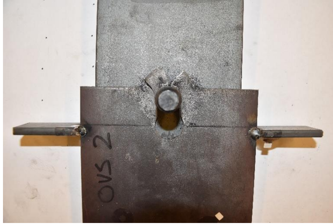
Figure 23: Photograph of specimen OVS2 after testing
