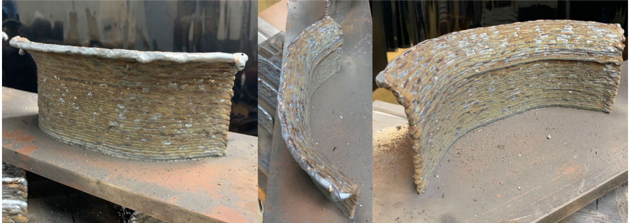
Figure 5.8: Views of the as built extended quarter bowl geometry produced using the new path planner software and methodology. The entire part planning takes less than a few hours including contour generation, path planning automatic NGA orientation calculations, and welding parameter assignments with KRL generation in Ocotopuz.
