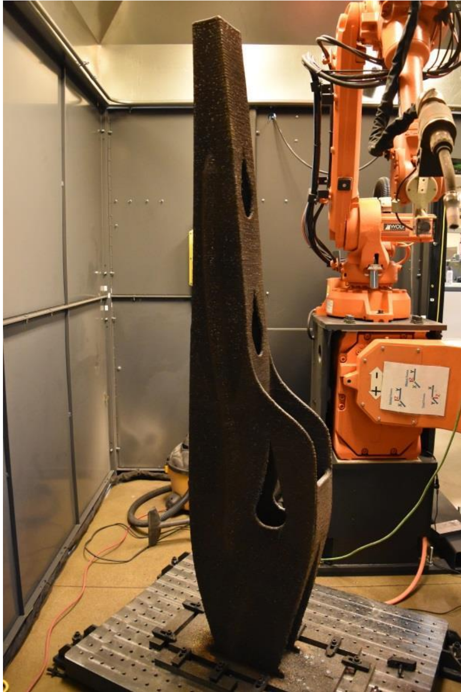
Figure 1.1: As-built excavator arm from [56] showing a large scale AM part using a WAAM system.
