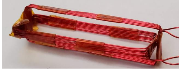
Fig. 3.18. A prototype of receiving coils.
