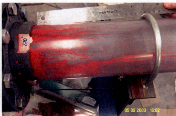
Figure 4-13. Exit Duct 270°, Aft 20 % Porous-Cell Honeycomb
