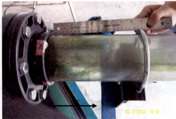
Figure 4-16. Exit Duct 270°, Aft 30% Porous-Cell Honeycomb
