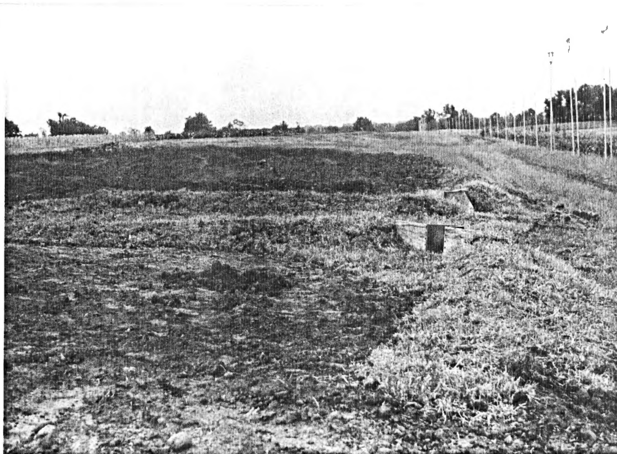
Figure 7. Test plots used to evaluate the effectiveness of diking in reducing water runoff and soil loss.
