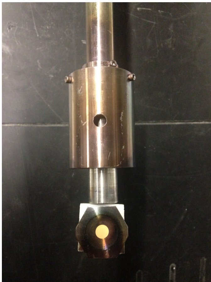
Figure 3.5: Detail of the QCM Teflon holder with shield to allow exposure of crystal only (shield slid upward).
