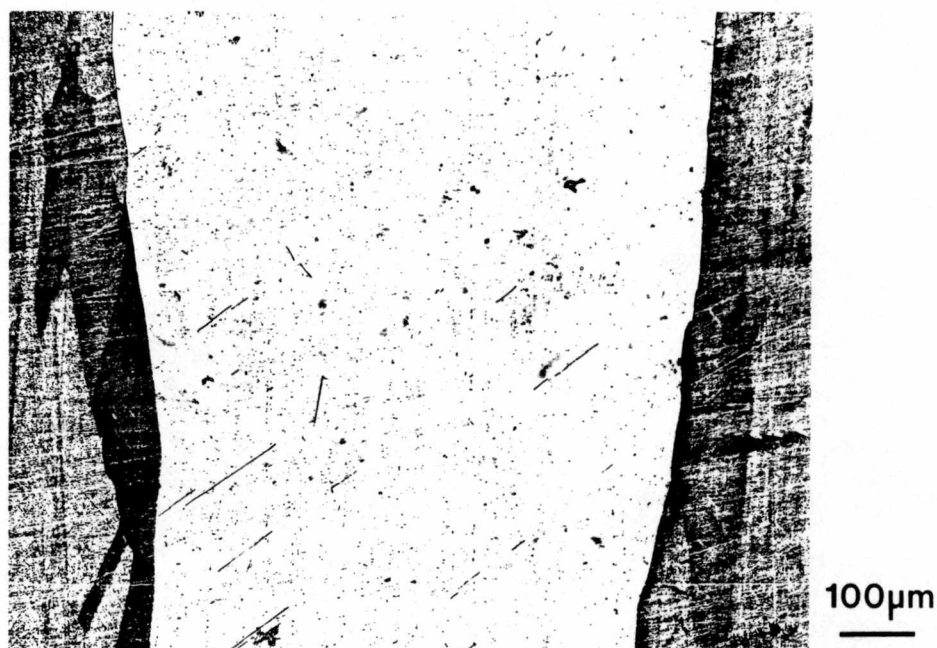
Figure 42. Directionally cast optical microstructure of Ti-54.1at%Al alloy showing single phase \gamma . N impurity content for the processed bar <40ppm.
