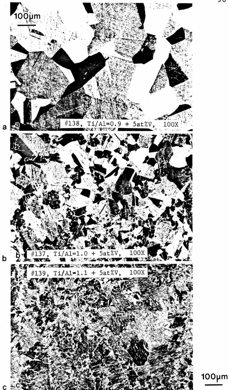
Figure 48. Optical microstructures of TiAl+5at%V with a varying Ti/Al ratio. a) Ti/Al=0.9 b) Ti/Al=1.0 c) Ti/Al=1.1
