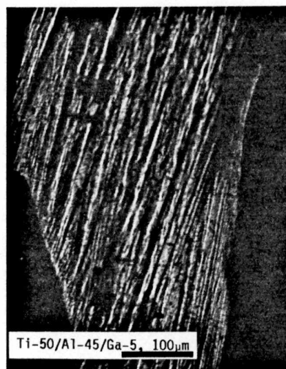
Fig. 6. Wavy slip in bulk specimen deformed 7.7% in compression.
