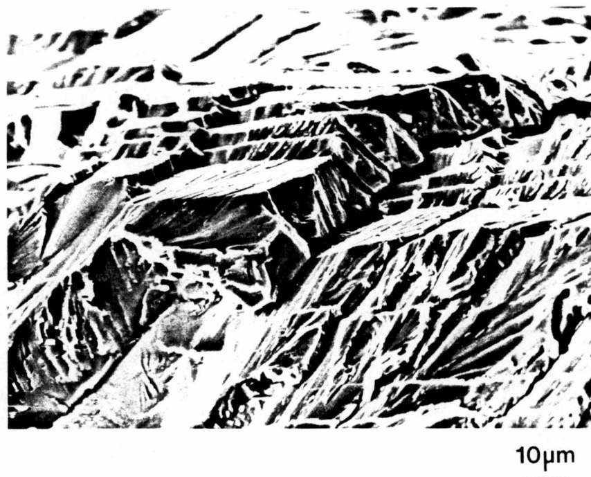
Figure 95. SEM oblique view of layered \{111\} plane fractures indicating the large included angle.
