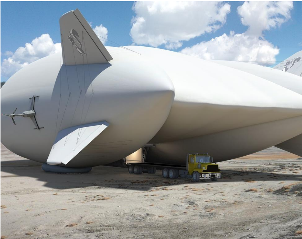
Figure 2.3. Lockheed Martin’s LMH-1 demonstrates its ability to unload cargo at truck bed height. [28]
