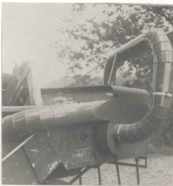
Figure 12. Main Duct Support
