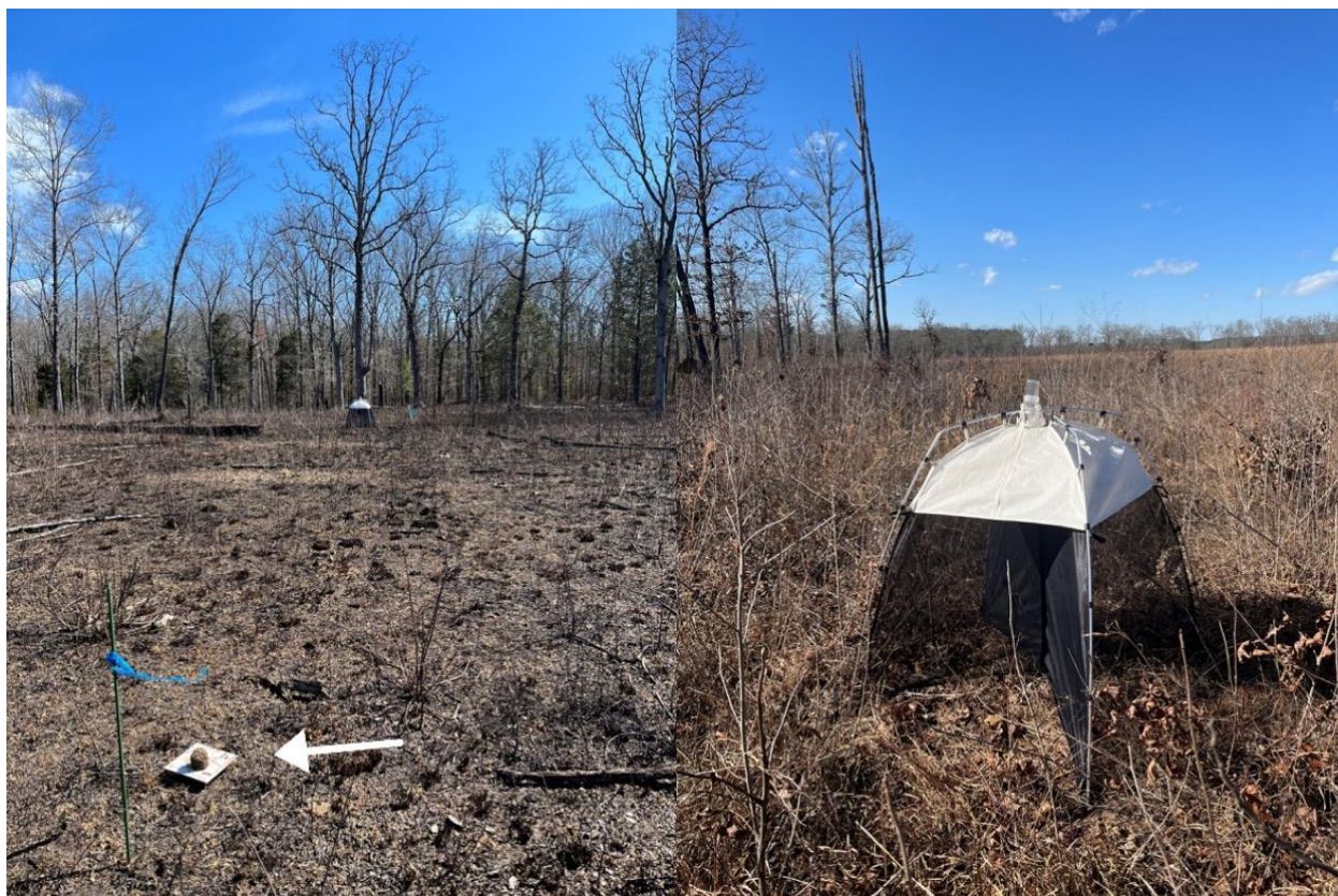
Figure 4: Pitfall trap (left) placed in a transect near SLAM (Sea -Land- Air Malaise) trap (right), Arnold Air Force Base, 2023.
