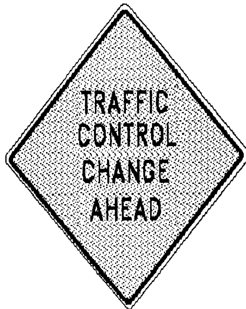
Figure 7 - Traffic Control Change Ahead Sign Oregon Department of Transportation
