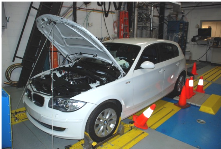
Figure 3.1 BMW 120i lean gasoline vehicle on chassis dynamometer at ORNL.
