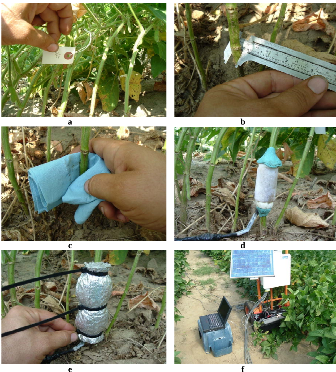
Figure 4.3. Use of Dynamax Flow32 System (fitting Dynagauges to soybean stem): a) each plant marked with durable tag for later identification, b) stem diameter measured and recorded, c) stem cleaned of dirt and debris, d) Dynagauge sensor placed around stem with top and bottom sealed with adhesive putty to prevent water and insect infiltration, e) insulating bubble wrap foil placed around Dynagauge (3 layers) and held in place with cable ties securely but with only light pressure, f) part of the Dynamax Flow 32 Sap Monitoring System setup as used in the field experiment showing the attachment to an upright cart for greater mobility, deep cycle marine battery and data link cable inside tool box at bottom, and portable computer for uploading program parameters and collecting data.
