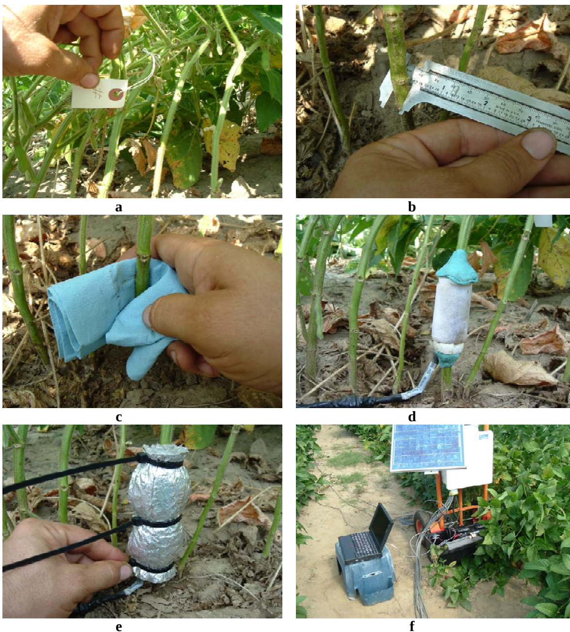
Figure 3.3. Use of Dynamax Flow32 System (fitting Dynagauges to soybean stem): a) each plant marked with durable tag for later identification, b) stem diameter measured and recorded, c) stem cleaned of dirt and debris, d) Dynagauge sensor placed around stem with top and bottom sealed with adhesive putty to prevent water and insect infiltration, e) insulating bubble wrap foil placed around Dynagauge (3 layers) and held in place with cable ties securely but with only light pressure, f) part of the Dynamax Flow 32 Sap Monitoring System setup as used in the field experiment showing the attachment to an upright cart for greater mobility, deep cycle marine battery and data link cable inside tool box at bottom, and portable computer for uploading program parameters and collecting data.
