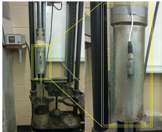
Figure 3: Accelerometer installed on the impact hammer.
