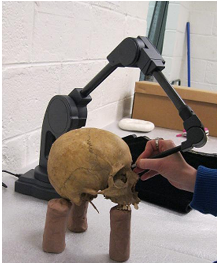
Figure 7. Digitizing of cranial landmarks using Microscribe.
