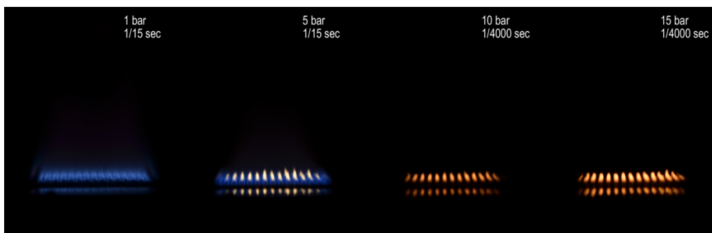
Figure 2.7: Effect of pressure on the Hencken flame.
