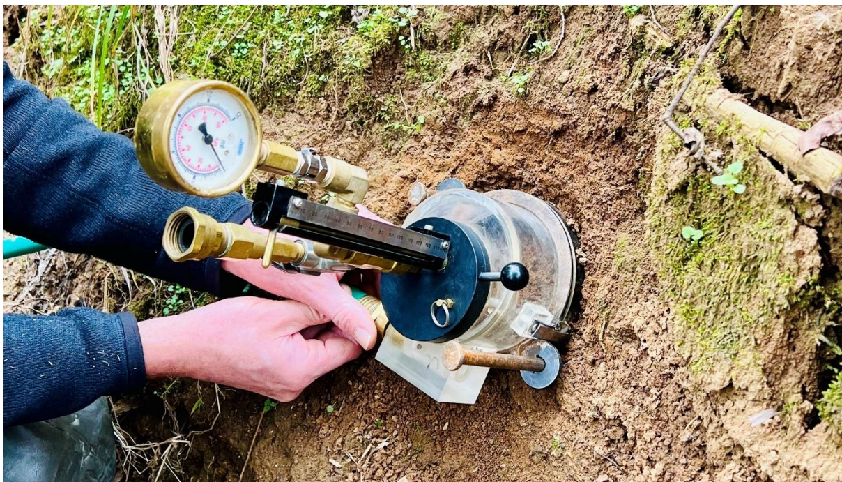
Figure 4-2 The JET Device installed at the bank of Conner Creek, Knox County, TN
