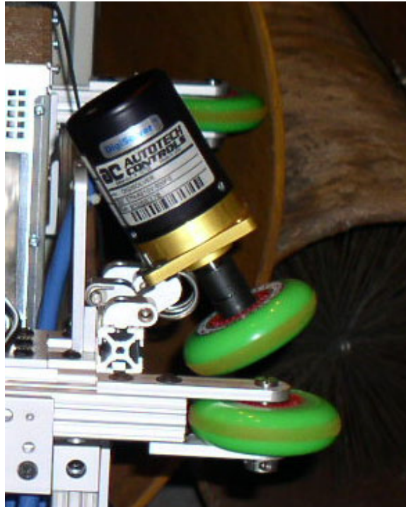
Figure 2.5: The spring loaded resolver mount is shown here. Also visible in this image are the rust “stains” that give an indication that the resolver wheel does not roll on its maximum circumference (compare the rust strips on the guide wheels to the rust strip on the resolver wheel).
