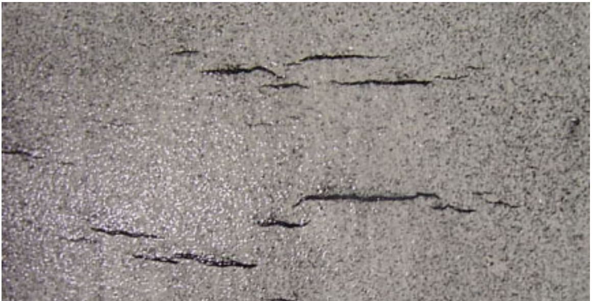
Figure 1.3: Color contrast MPI image of an SCC colony from a decommissioned natural gas pipeline. The SCC colony is 2\frac{8}{10} inches long and approximately 1\frac{2}{5} inches wide.
