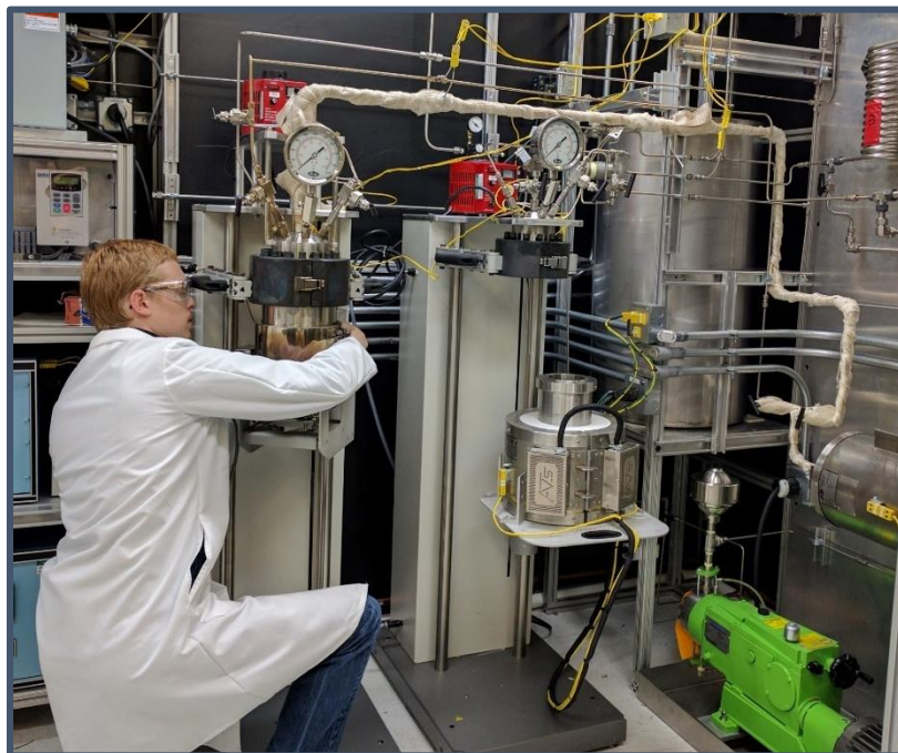
Figure 3.2: Images of the HCL water loop (excluding the DI water section) with Dr. Stephen Raiman and the author operating the loop.
