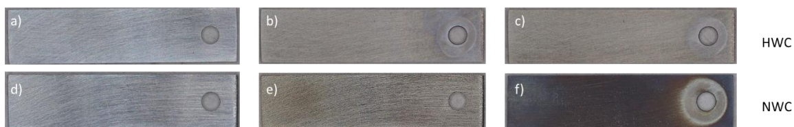
Figure A. 5: Pictures of pure Cr at a) 0h, b) 200h, and c) 400 h of exposure in a BWR-HWC (288°C, 150ppb H 2 ) environment and d) 0h, e) 200h, and f) 400h of exposure to the BWR-NWC (288°C, 2ppm O 2 ) environment.
