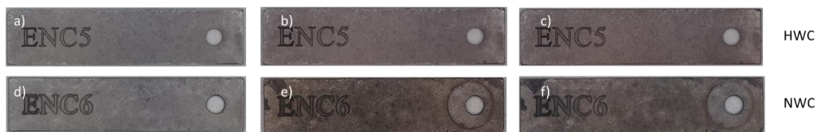
Figure A. 8: Pictures of pure CrN-coated CVD SiC at a) 0h, b) 200h, and c) 400 h of exposure in a BWR-HWC (288°C, 150ppb H 2 ) environment and d) 0h, e) 200h, and f) 400h of exposure to the BWR-NWC (288°C, 2ppm O 2 ) environment.
