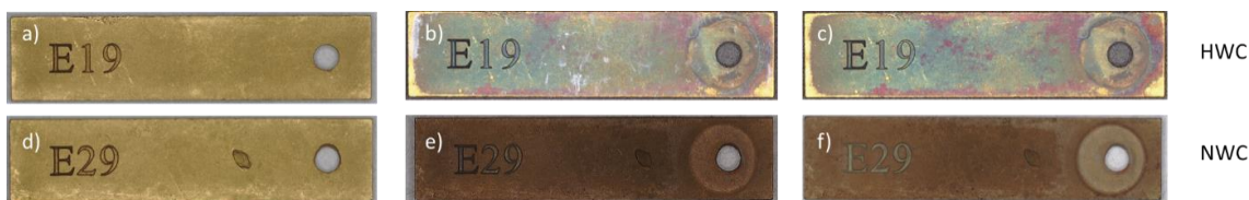
Figure A. 11: Pictures of TiN-coated CVD SiC at a) 0h, b) 200h, and c) 400 h of exposure in a BWR-HWC (288°C, 150ppb H 2 ) environment and d) 0h, e) 200h, and f) 400h of exposure to the BWR-NWC (288°C, 2ppm O 2 ) environment.
