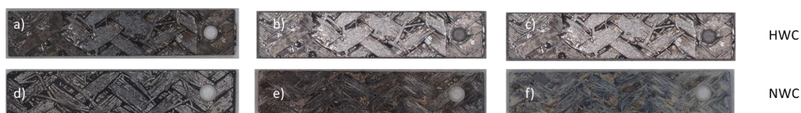
Figure A. 3: Pictures of pure CMC SiC from NGNP at a) 0h, b) 200h, and c) 400 h of exposure in a BWR-HWC (288°C, 150ppb H 2 ) environment and d) 0h, e) 200h, and f) 400h of exposure to the BWR-NWC (288°C, 2ppm O 2 ) environment.
