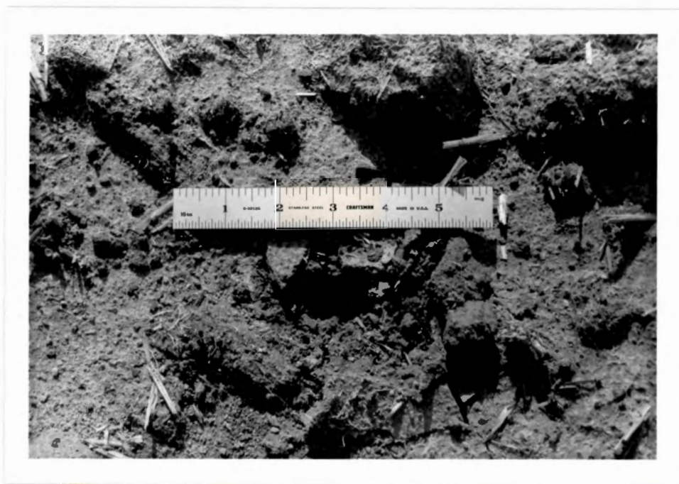
FIGURE 28. Width of single hole formed by probe indicated with scale having traditional English units.
