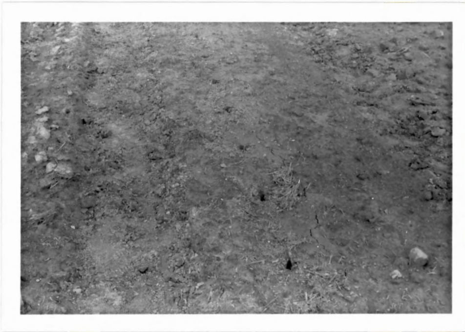
FIGURE 26. Row of seven holes in soil demonstrating pattern of soil disturbance resulting from probe operation.
