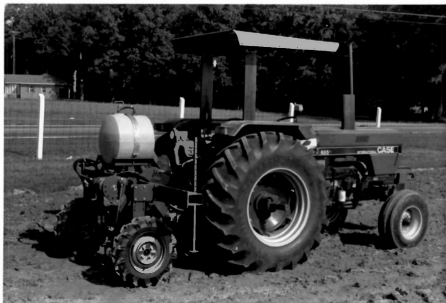
FIGURE 23. Side view of injector hitched to Case-IH 685 tractor.
