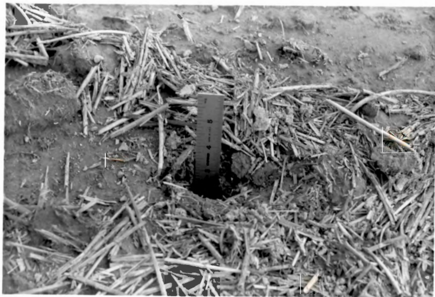
FIGURE 27. Depth of single hole formed by probe indicated with scale having traditional English units.
