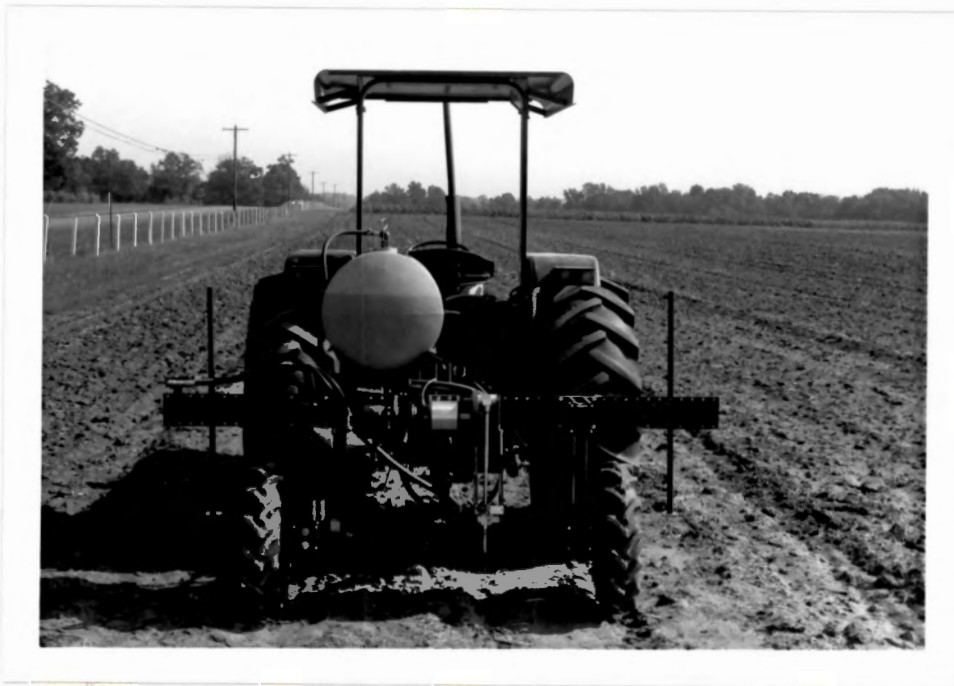
FIGURE 24. Rear view of injector hitched to Case-IH 685 tractor.
