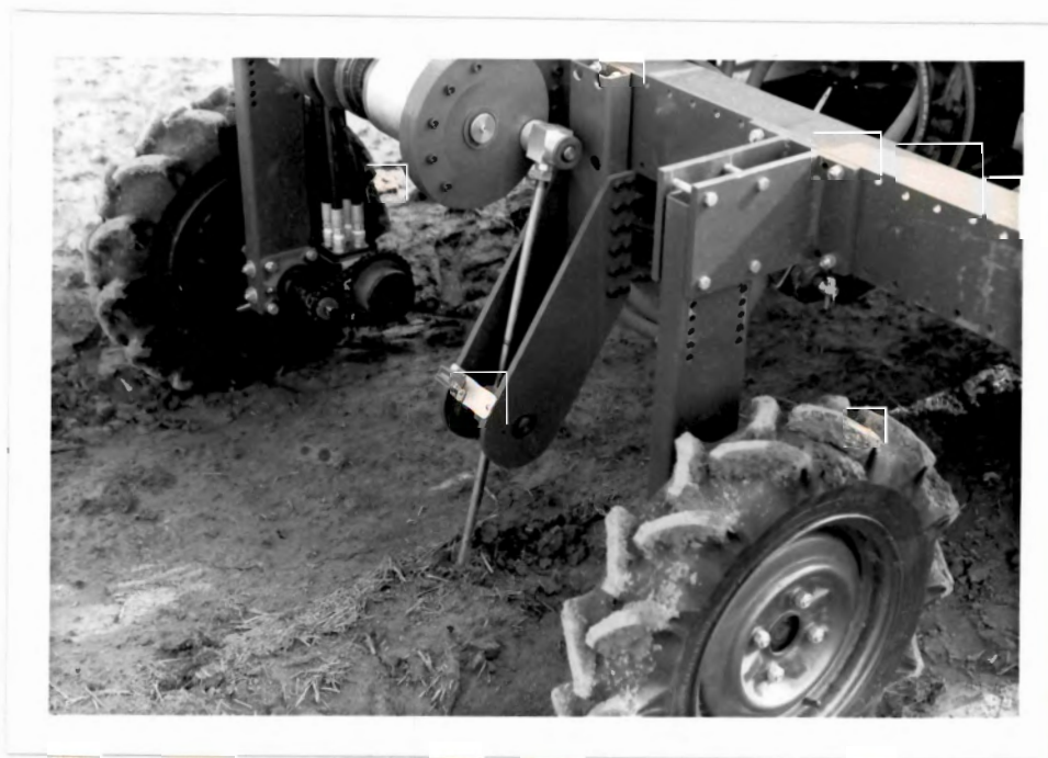
FIGURE 25. Probe exiting soil during field evaluation of injector.
