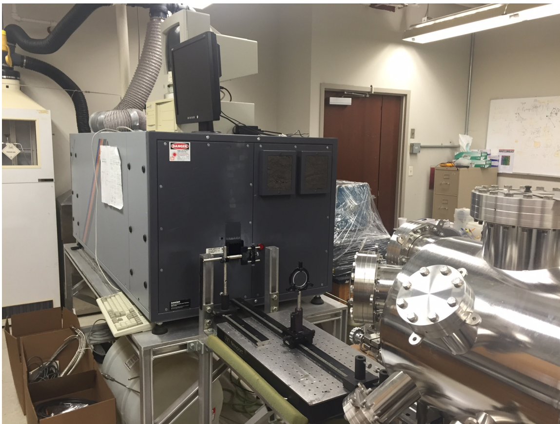
Figure 2.9. Lambda-Physik LPX300cc KrF Excimer Laser with optical table, converging lens, and sample chamber, in the foreground. The wavelength of the laser is 248 nm and the experimental energy range, depending on the experiment, was E = 150 - 250 \text{ mJ/cm}^2 .
