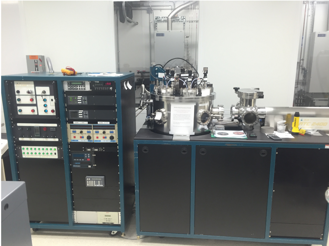
Figure 2.7. AJA International ATC2000 Sputtering System
