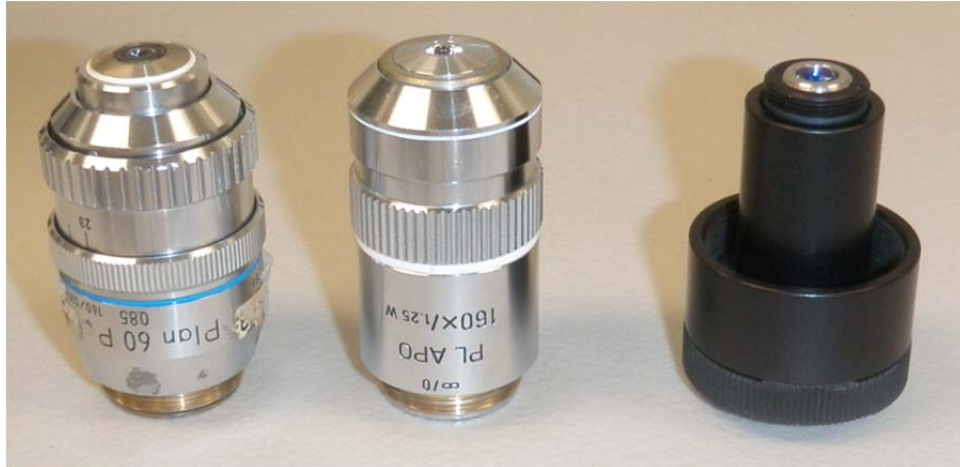
Figure 3.3(b). A photograph of the lenses used for laser machining: left: 60 \times ; middle: 160 \times ; right: 60 \times aspheric lens.
