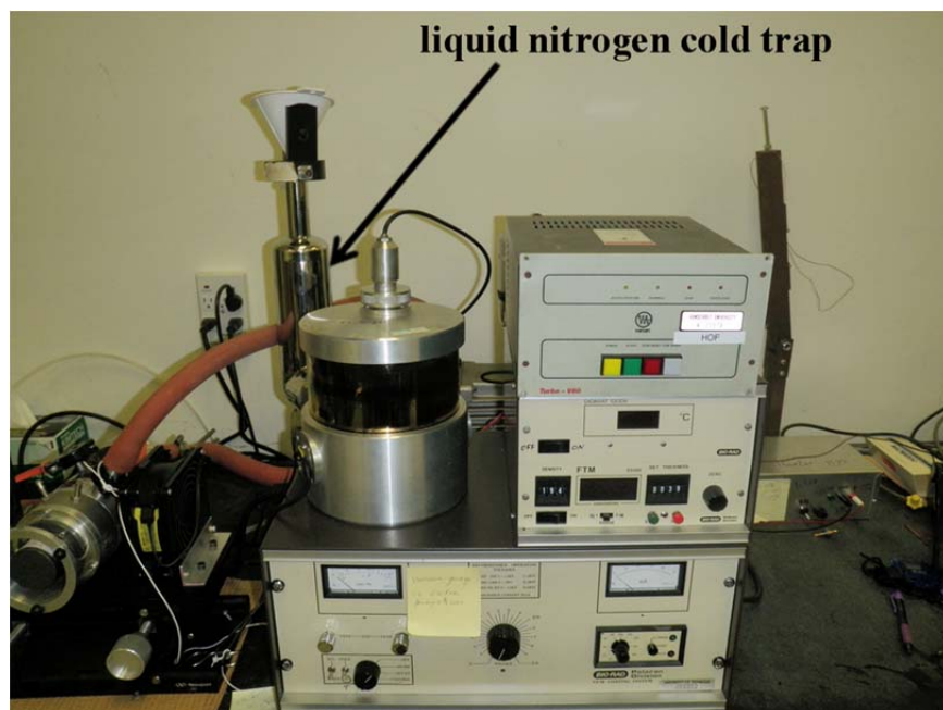
Figure 3.5.1. A photograph of the sputtering machine modified with a liquid nitrogen cold trap to coat gold, platinum, and palladium on polymer nanowires at cryogenic temperatures.
