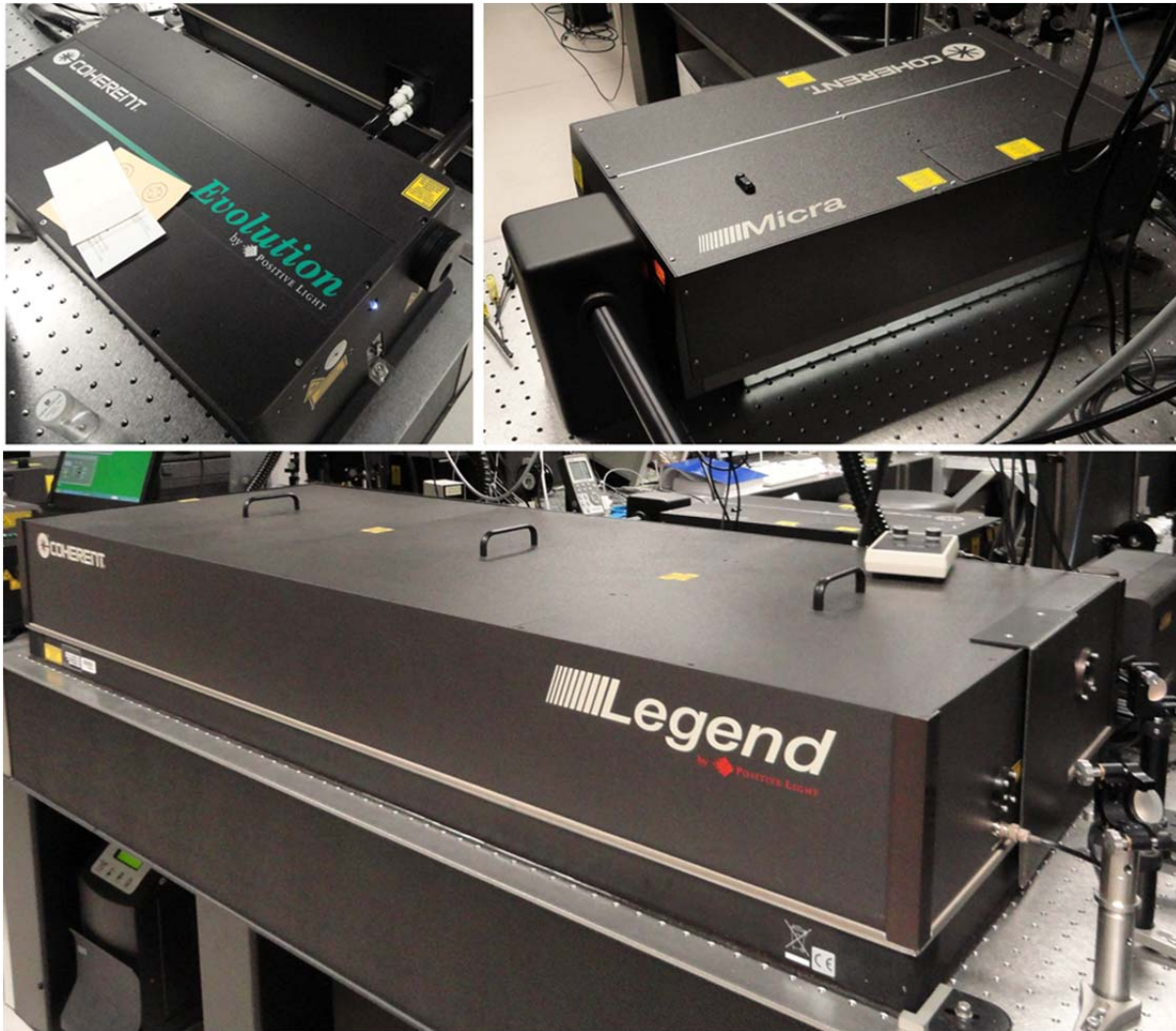
Figure 5.3(b). A photograph of the amplified femtosecond laser set-up used for aspheric lens machining of fused silica. The output is a train of 1 kHz amplified femtosecond laser pulses of wavelength \sim 800 nm, temporal length 40 fs, and maximum pulse energy \sim 1.6 mJ.
