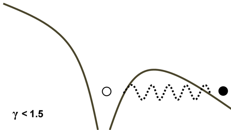
Figure 2.1.1. Ionization by tunneling of the bound electron due to suppression of the potential barrier caused by the strong electric field of the laser beam. This is called tunneling ionization or optical field ionization. This graph represents the potential (electrostatic) energy of the electron in the electric field of the laser. (empty circle = hole; solid circle = electron; the solid line is a graph of the Coulomb potential energy of an electron (y-axis) as a function of the radial position (x-axis) of the electron.)
