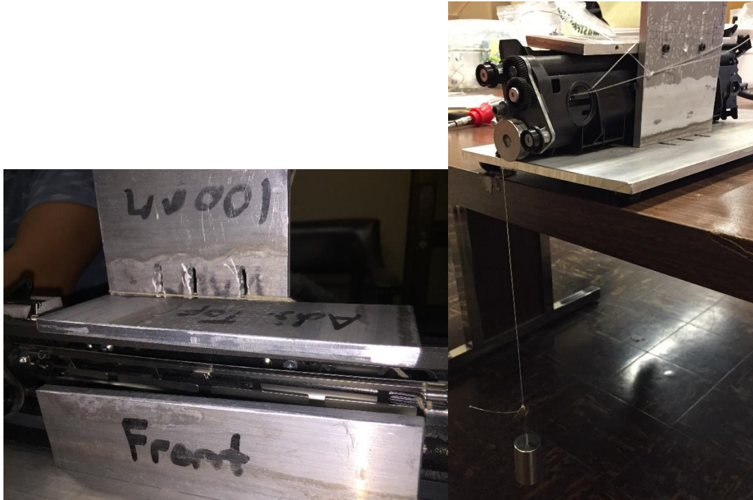
Figure 5. Gear Failure Test Apparatus and Loading Flywheel
