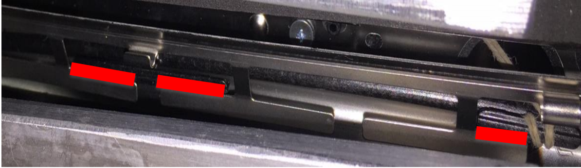
Figure 10. Additional Problem: Interference with Metal “T’s” Due to Extreme Deflection of Agitator Shaft (Marked by Red Zones)
