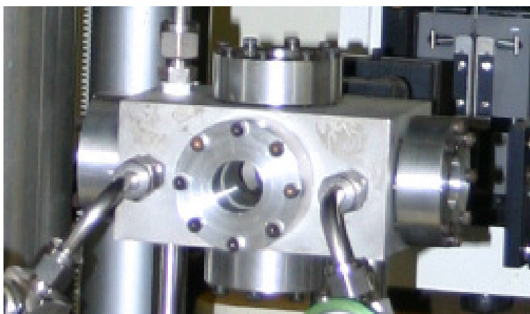
Figure 4.2: Photograph of the high pressure sample vessel with the spectrometer slit in the background.
