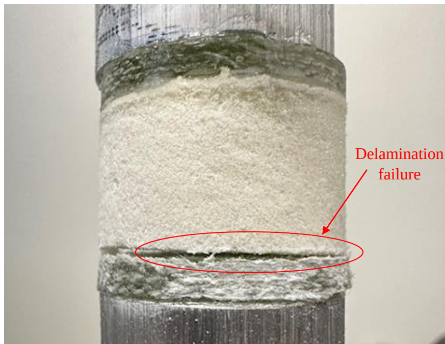
Figure 61. Failure by delamination in the Prisma sandwich under a “flatwise” tensile test (ASTM D7291).
