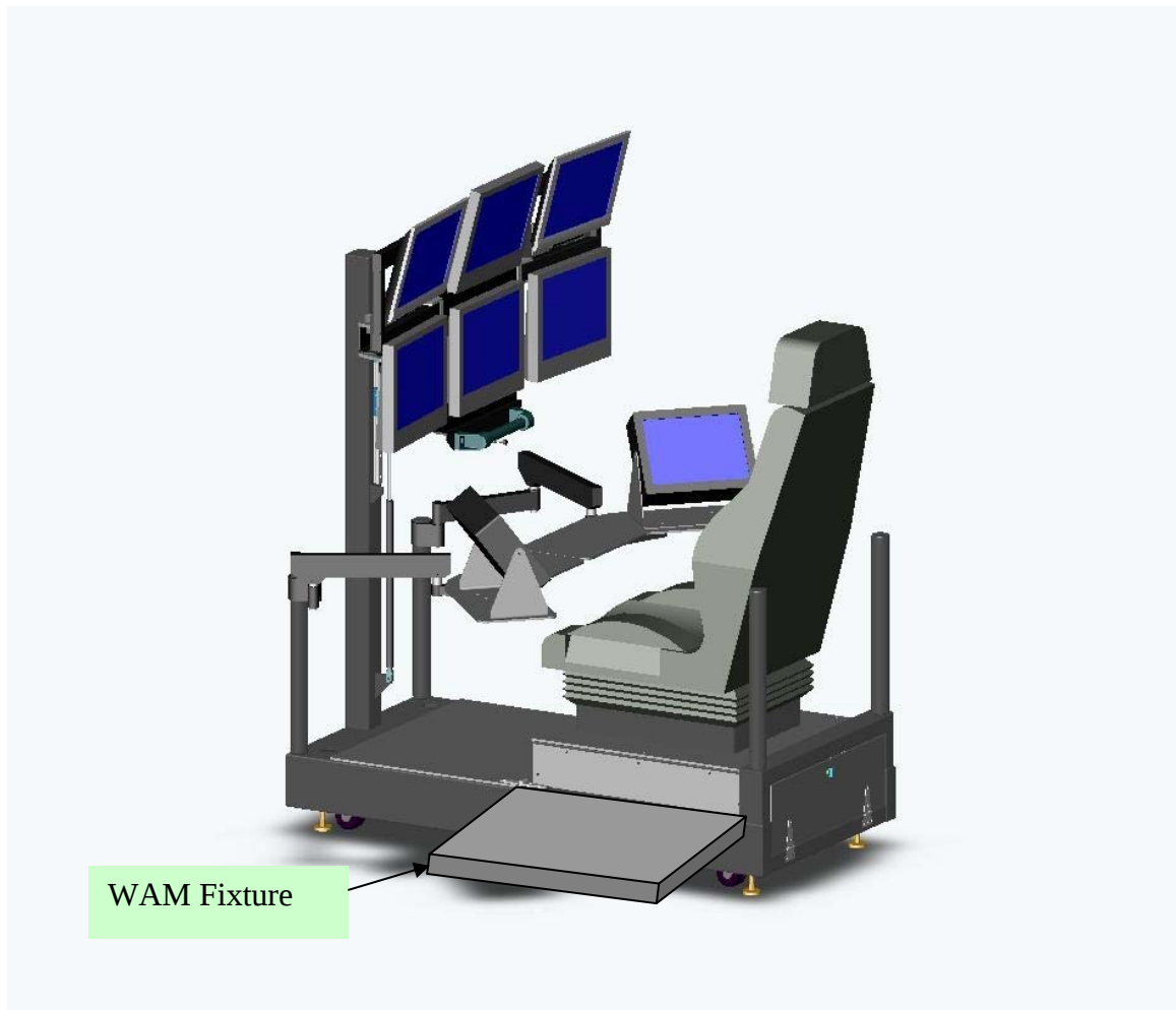
Fig 4.5. Compact Remote Console
