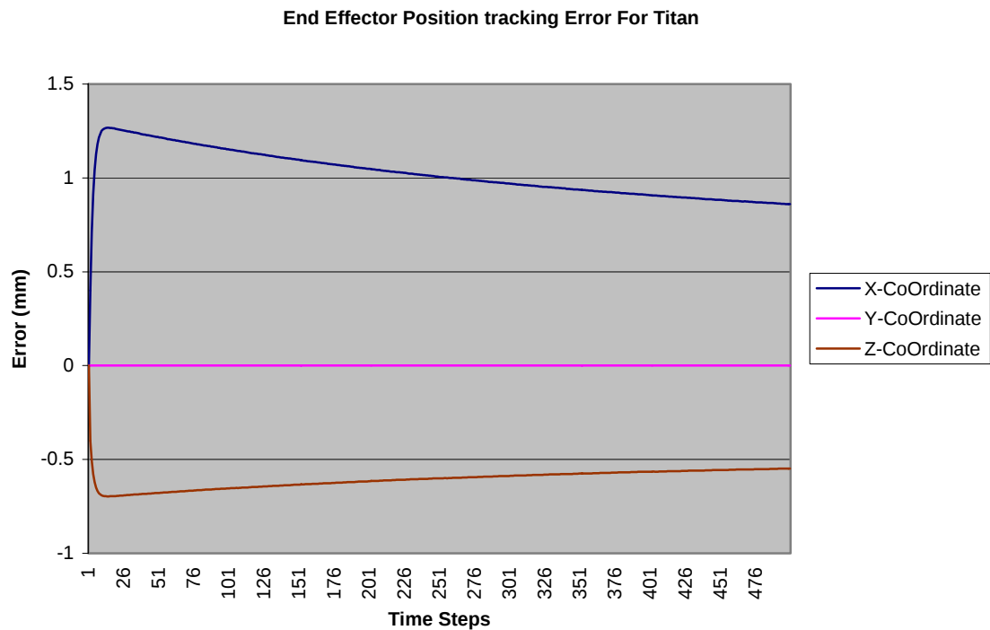
Fig 6.25 End Effector position tracking error for a different trajectory
