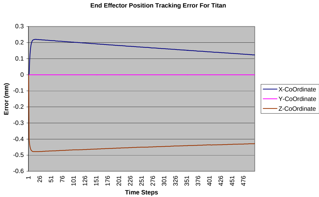
Fig 6.24 End Effector position tracking error for Titan
