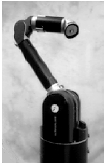
Fig 1.2 Master manipulator WAM
