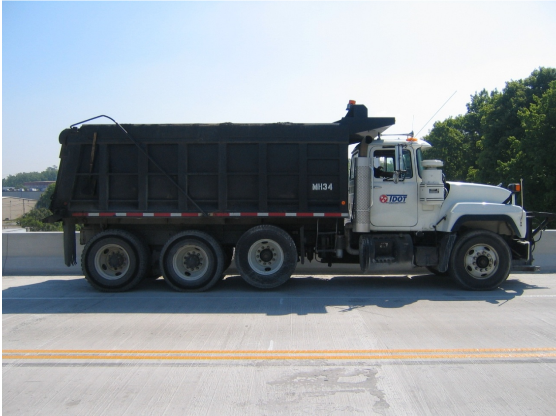
Figure 14: Typical scene of a controlled load test (Massman Dr Bridge). Note the white line perpendicular to the double yellow line marking the position of the front axle when the truck was stopped at position D.
