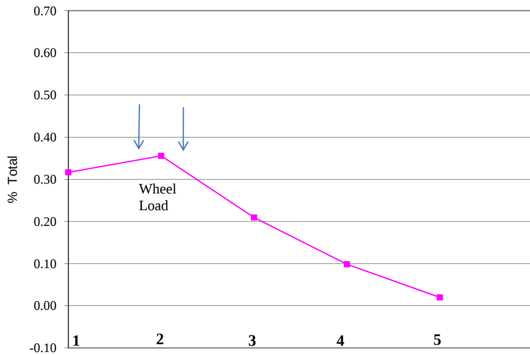
Figure 21: Massman Drive Load Distribution Factors for Load Over Girder 2 (Positive Moment).
