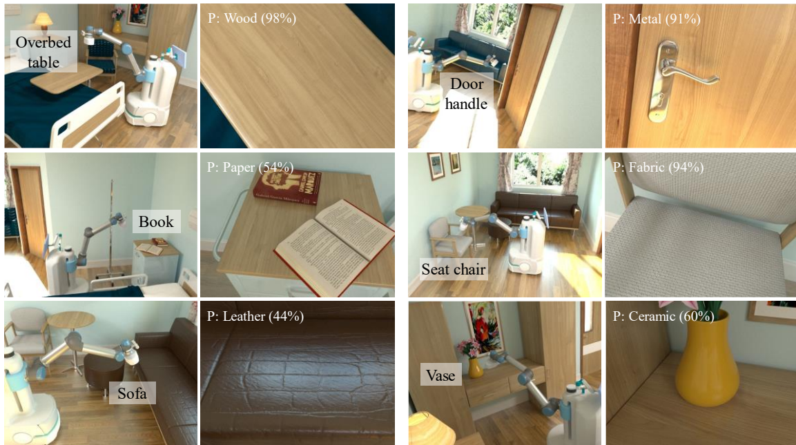
Figure 5.9. Example results of material classification on images captured by the robot. P: predicted material (confidence value in parentheses)
