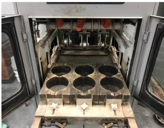
(c) Traditional asphalt mix mold
