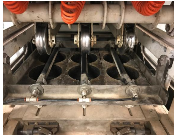
(b) Loading wheels and rubber hoses
