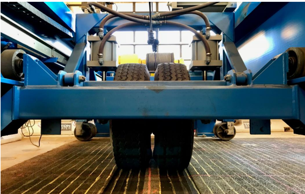
(b) Loading dual-wheel assembly
