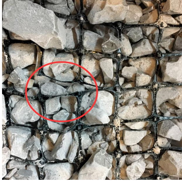
Figure 3.9. Deformation and breakage of biaxial geogrids in AGG2 (19 - 25 mm)
