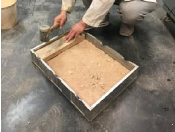
(a) Base course materials compaction
