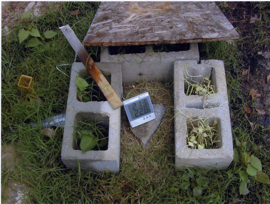
Figure 12. Thermometer structure- created with cement block and a plywood cover to protect the mechanics of the thermometers from direct sunlight and rain. The outdoor sensor is attached to the small wood stake. Structures were exactly the same at the sun and shade locations.
