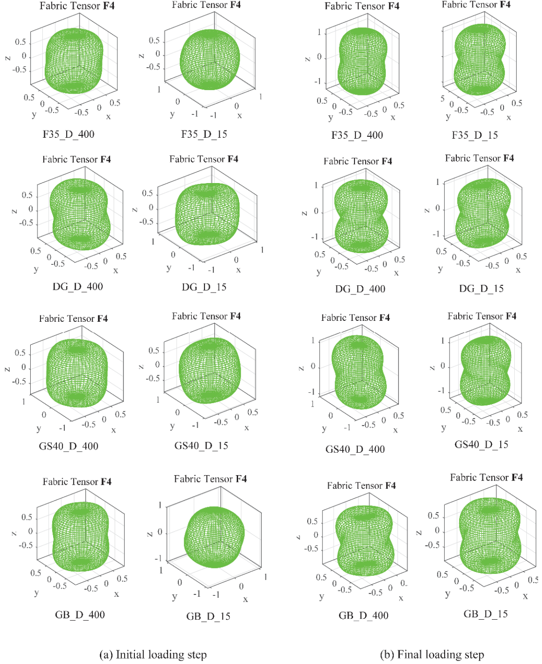
Figure 20. Comparison between \mathbf{F4} representation surfaces of global contact unit normal vectors of dense 400 kPa versus dense 15 kPa experiments at (a) initial and (b) last loading stage.
