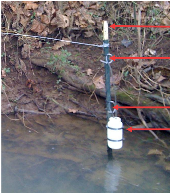
Figure 5: The typical passive sampler setup. The only time this setup was changed was if the stream bedrock prevented the installation of a fence post.
