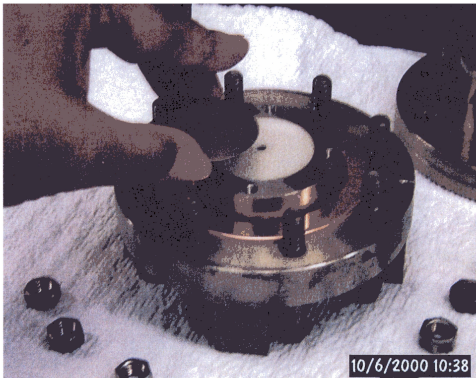
Figure 3.3. Specimen chamber with compression shim being placed on foam specimen.
