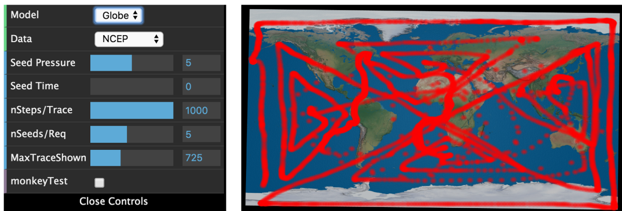
Figure 3.7: Left: UI controls of the tracing app (Section 3.3.1). Right: Monkey testing request locations. Each test makes 3,481 requests in 1 minute at roughly a rate of 60 requests/second. Each request includes 5 seeds for particle tracing.
