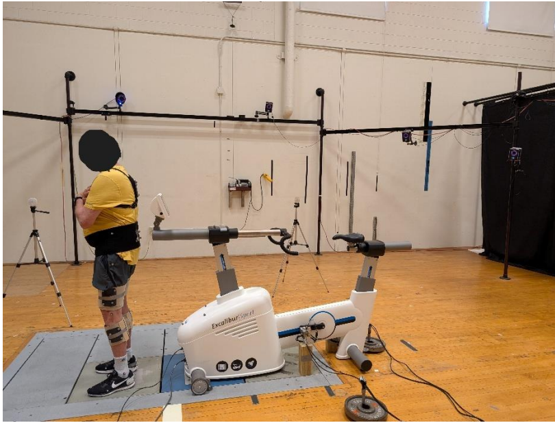
Figure 1: Data collection setup of ergometer, motion capture, and participant
