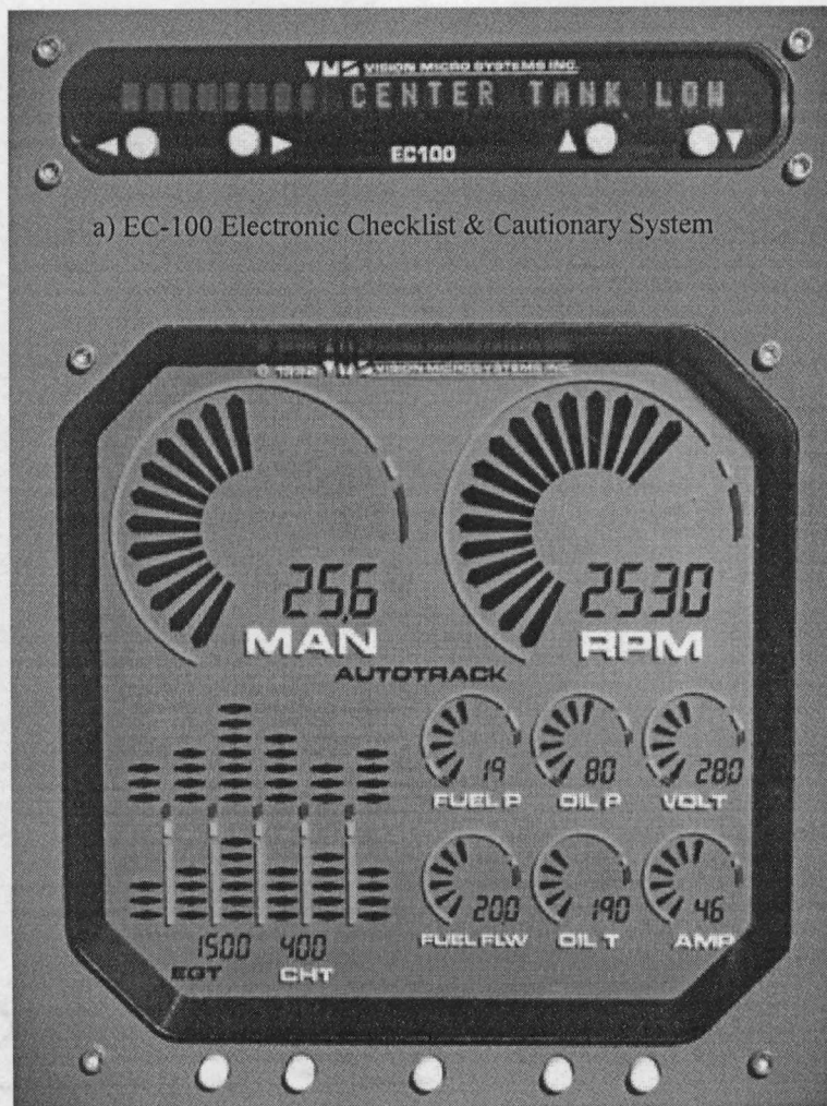
Figure A-11. Vision Microsystems Inc's VM1000 & EC-100 Engine Instrumentation Caution Advisory System.
