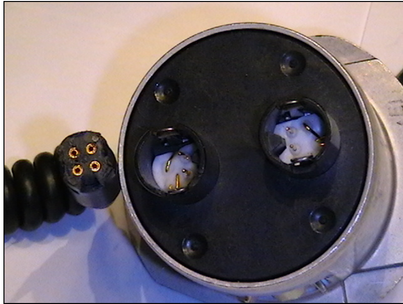
Figure 9 Bent Pins on FZU-48 Bomb Fuze Initiator Source: Author
