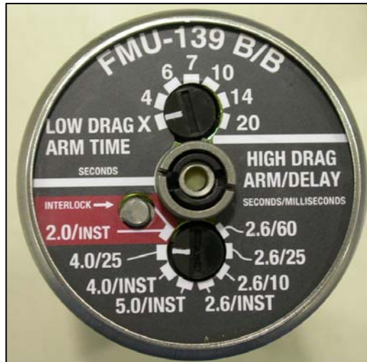
Figure 3 Faceplate of the FMU-139B/B Source: Precision Strike Weapons Bomb Systems Commodities
