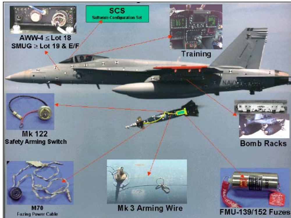
Figure 1 Major Components of the Fuzing System Source: Mr. Gary Evans, U.S. Navy
