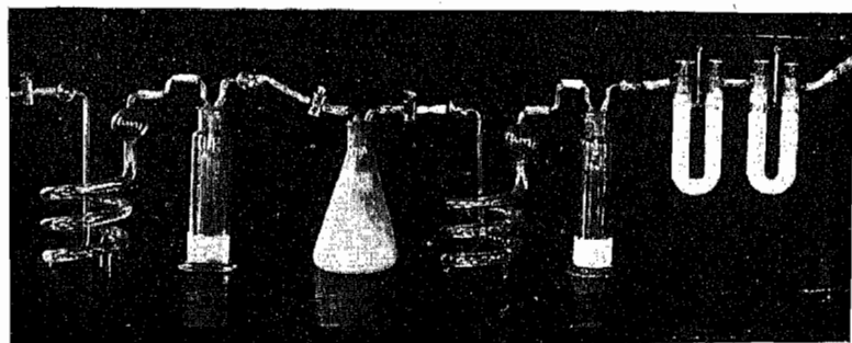
APPARATUS FOR MEASURING DECOMPOSITION OF SOIL CARBONATES
