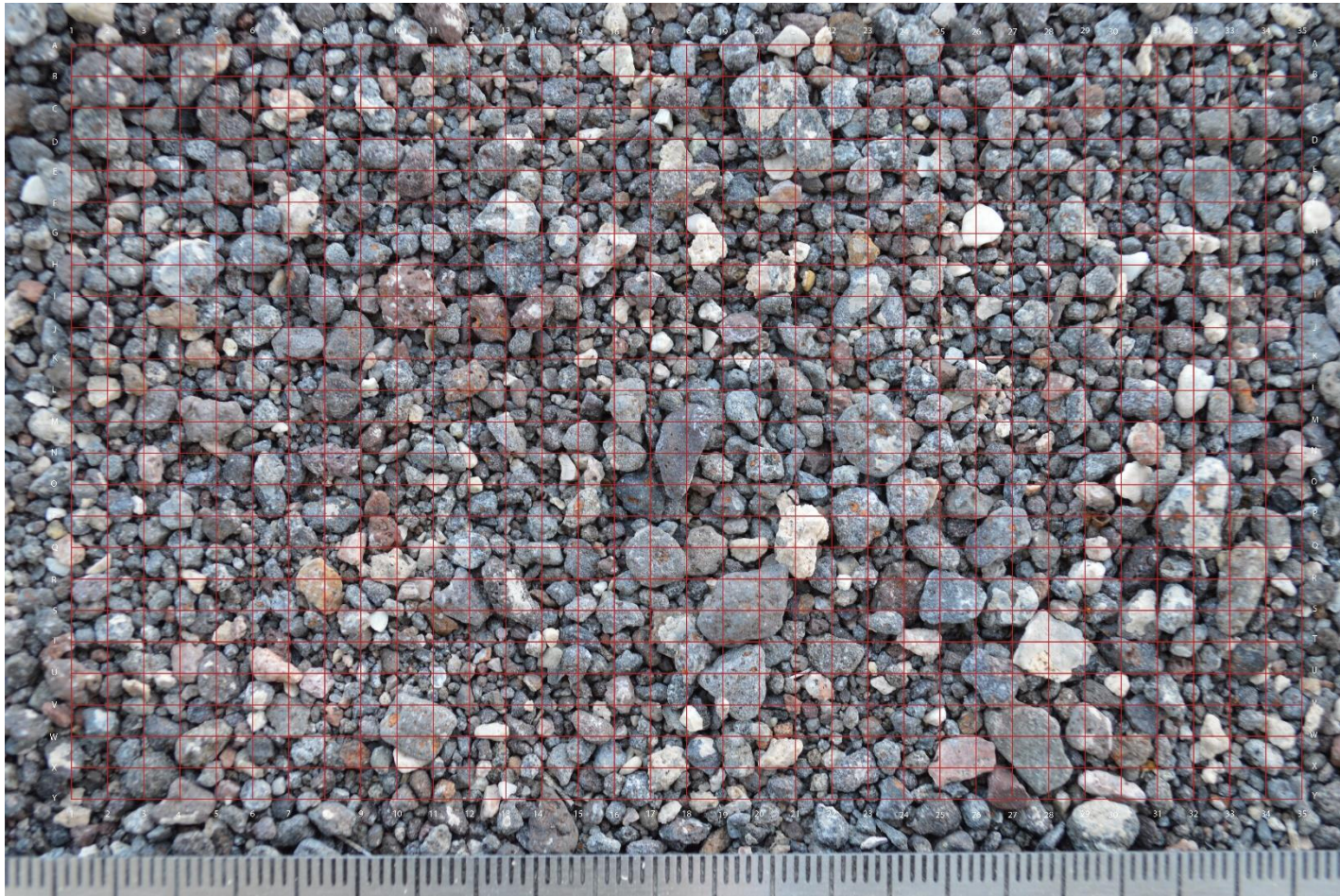
Figure A9: Image of fluvial sediment taken under even illumination at 19 \mu\text{m}/\text{pixel} image resolution.
