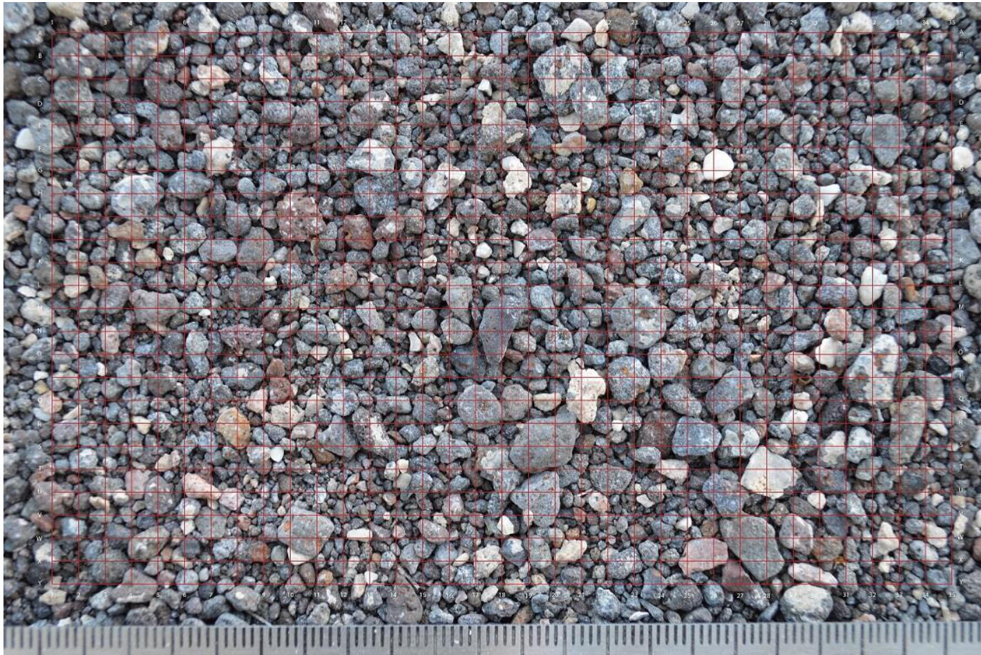
Figure A13: Image of fluvial sediment taken under even illumination and resampled to 100 \mu\text{m} /pixel image resolution
