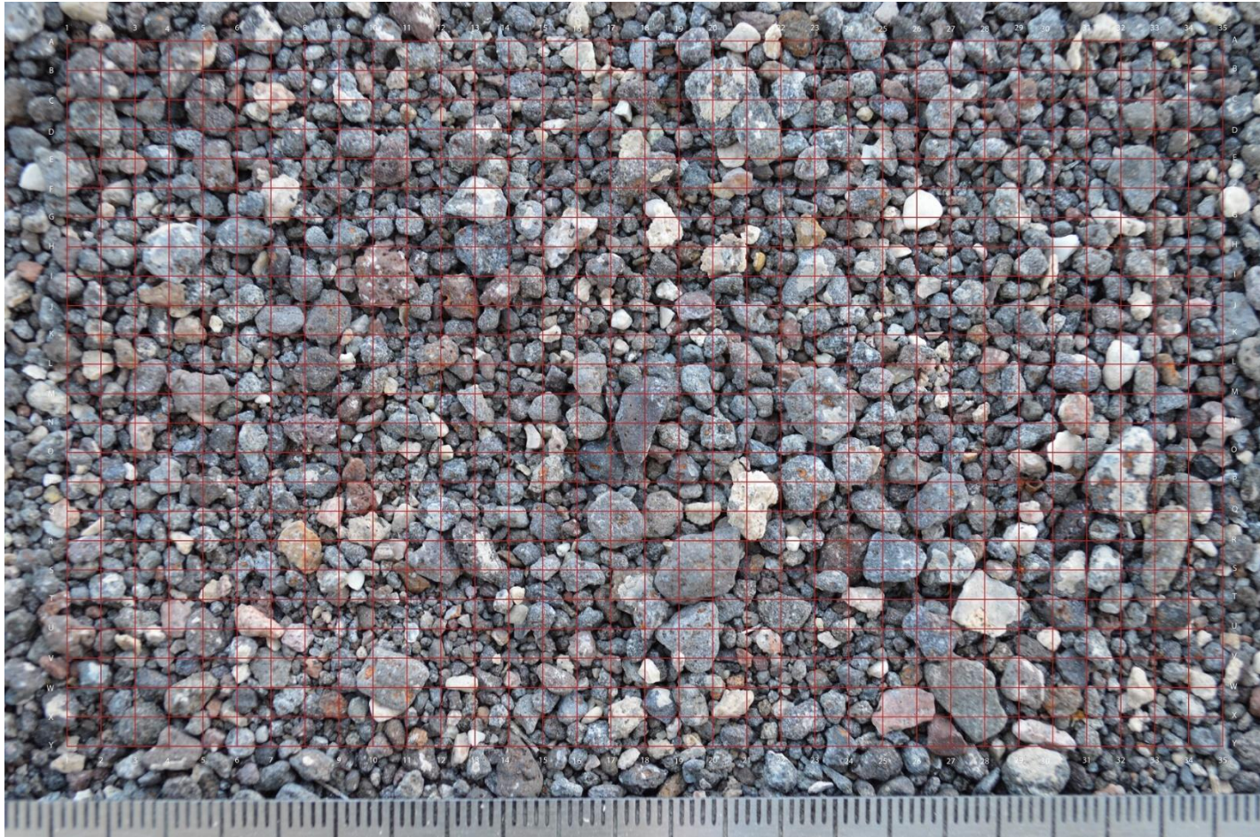
Figure A11: Image of fluvial sediment taken under even illumination and resampled to 60 \mu\text{m} /pixel image resolution.
