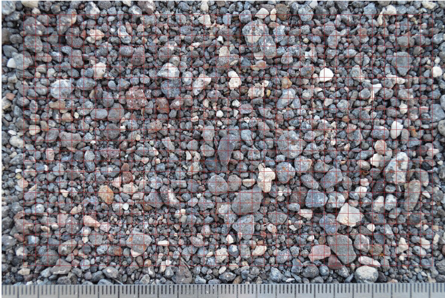
Figure A12: Image of fluvial sediment taken under even illumination and resampled to 80 \mu\text{m} /pixel image resolution.
