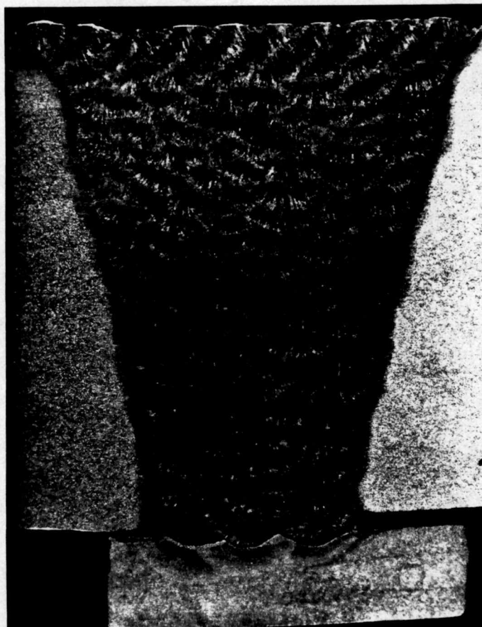
Figure 17. Macrograph of the shielded metal arc weld in PWHT (1050°F-25 hrs.) condition, 1.4X, 3HCl-2H 2 O-1H 2 O 2 etch.
