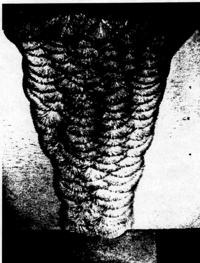
Figure 16. Macrograph of the submerged arc weld in as-welded condition, 1.4X, Hrubec's etch.
