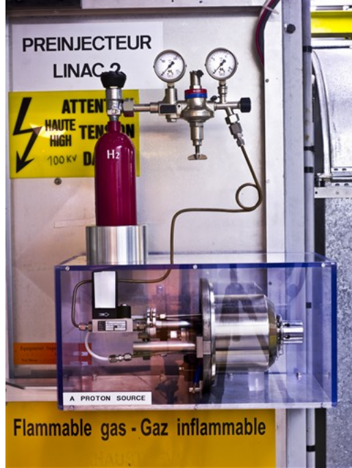
Figure 3.2: The source of protons for the LHC.
