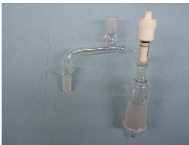
Figure 3 - 5 A picture of bent tee-shaped glassware
