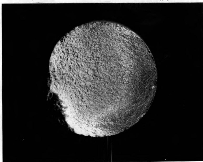
Figure 24. Photomicrograph of a D-8 Fracture Surface. Specimen Failed after 4.32 \times 10^6 Cycles; Applied Stress, 32730 psi ( 226 \text{ MN/m}^2 ) (50% of the YS). 8x.
