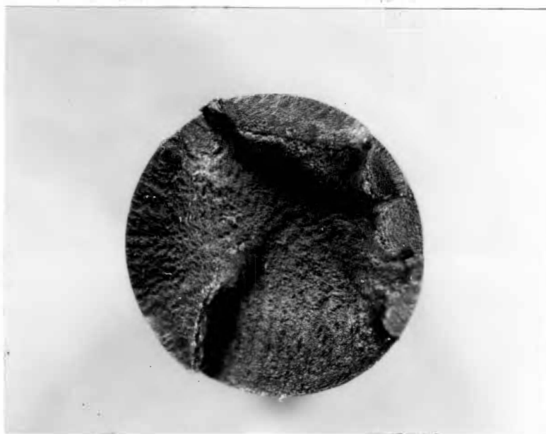
Figure 22. Photomacrograph of a D-8 Fracture Surface. Specimen Failed after 2600 Cycles; Applied Stress, 85199 psi ( 587 \text{ MN/m}^2 ) (129% of the YS) . 8x.
