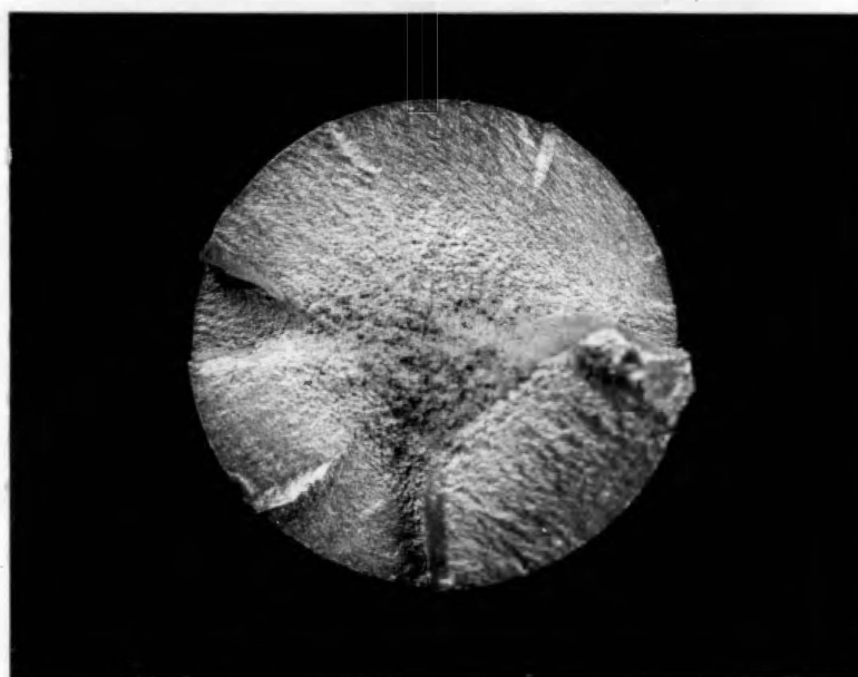
Figure 22. Photomacrograph of a D-8 Fracture Surface. Specimen Failed after 2600 Cycles; Applied Stress, 85199 psi ( 587 \text{ MN/m}^2 ) (129% of the YS) . 8x.
