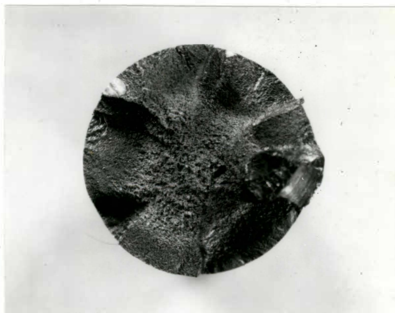
Figure 20. Photomicrograph of a D-1 Fracture Surface. Specimen Failed after 24700 Cycles; Applied Stress, 56211 psi ( 388 \text{ MN/m}^2 ) (84% of the YS). 8x.
