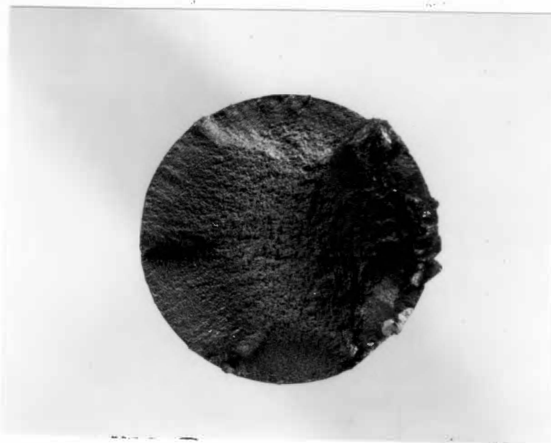
Figure 26. Photomicrograph of a D-24 Fracture Surface. Specimen Failed after 14200 Cycles; Applied Stress, 54995 psi ( 379 \text{ MN/m}^2 ) (91% of the YS) . 8x.
