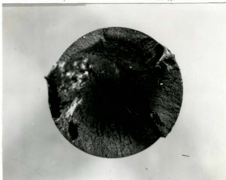
Figure 19. Photomicrograph of a D-1 Fracture Surface. Specimen Failed after 6800 Cycles; Applied Stress, 71004 psi ( 490 \text{ MN/m}^2 ) (106% of the YS). 8x.
