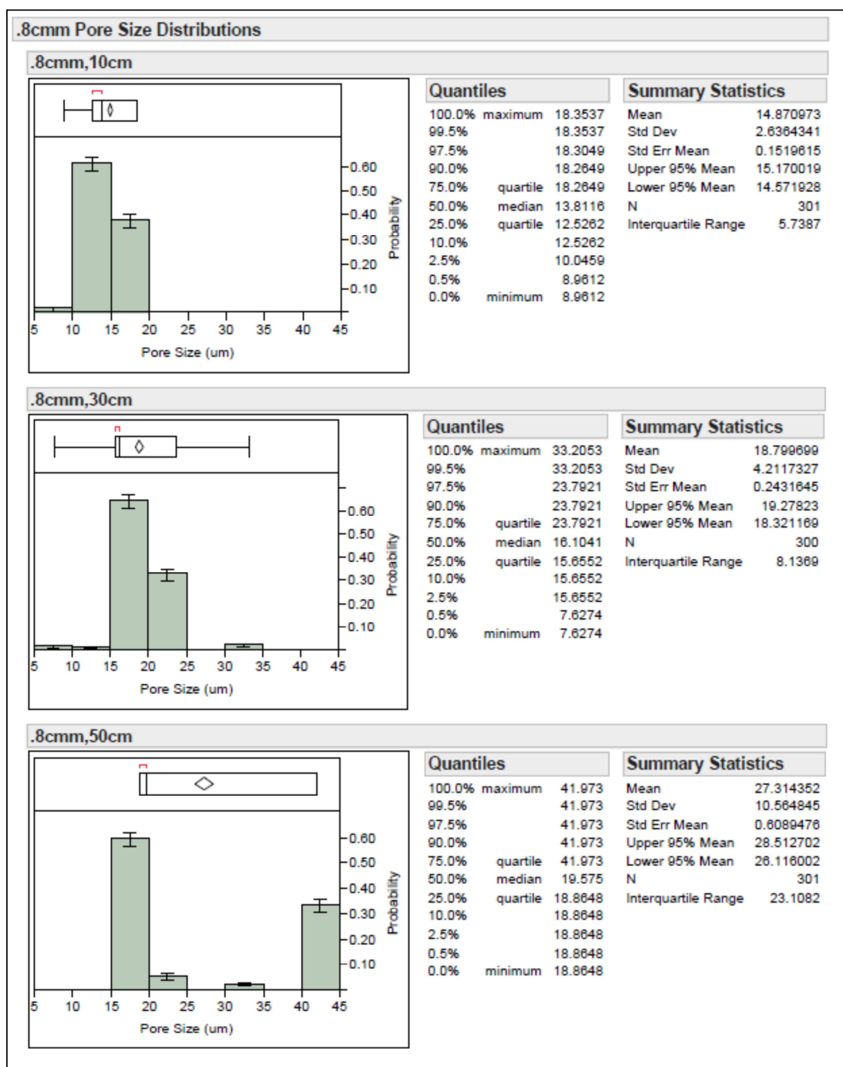
Figure 35. Pore Size distributions and statistics for nano-sized MB webs blown at 0.8cmm and collected at 10, 30 and 50cm
