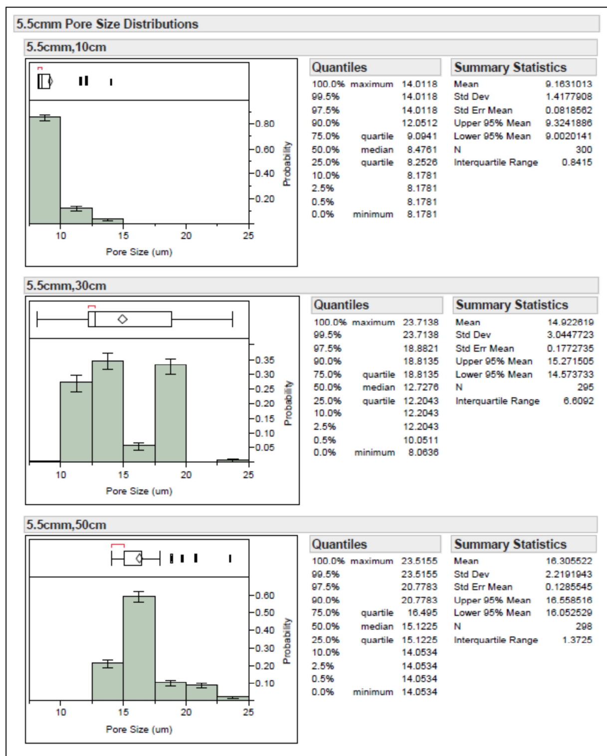
Figure 37. Pore Size distributions and statistics for nano-sized MB webs blown at 5.5cmm and collected at 10, 30 and 50cm
