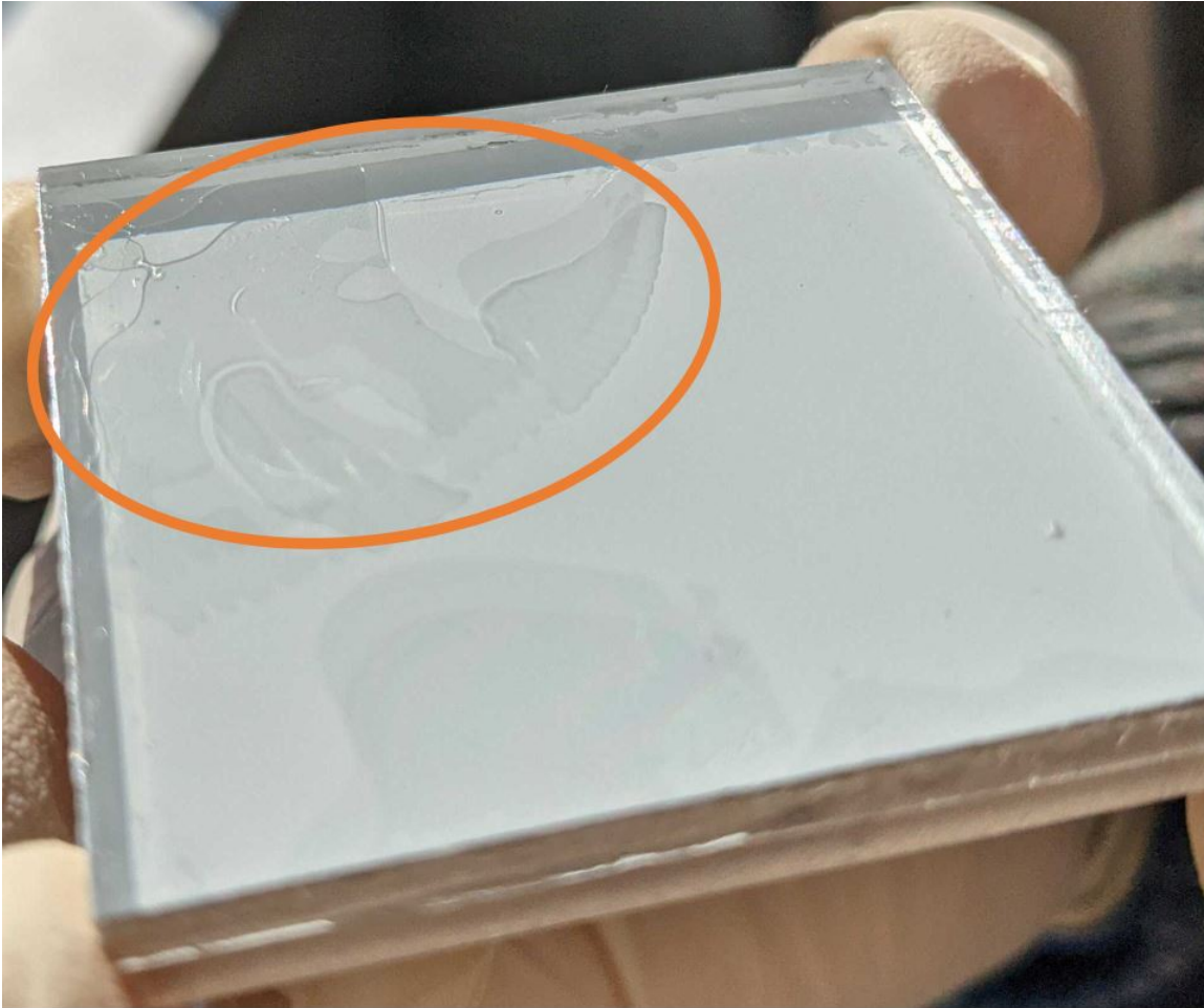
Figure 5.9: Optical distortion due to the separation of the light spreader and the scintillator (circled in orange).
