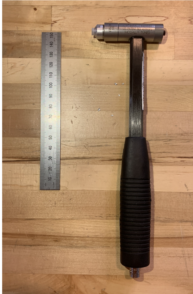
Figure 5: The modal hammer used in the experiment
