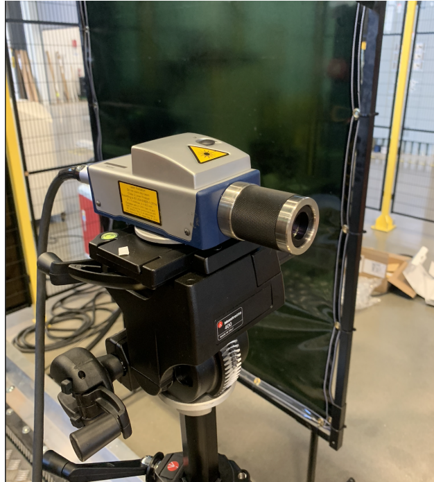
Figure 8: The laser Doppler vibrometer used to measure the low frequency tool-tip FRF
