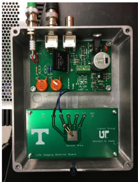
Figure 2.3.1. A) Custom enclosure containing the evaluation board and preamplifier, B) Secondary enclosure only containing the evaluation board
