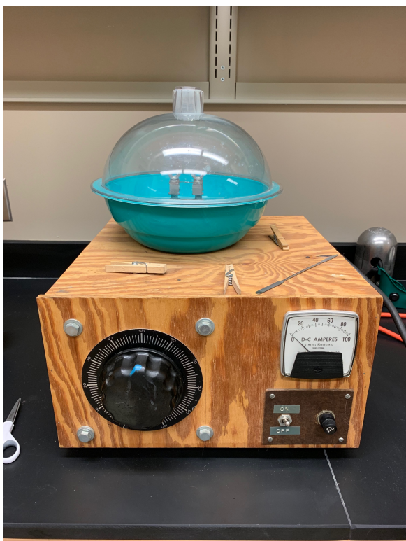
Figure 3.4 1 Instrument used to create glass beads for bulk analyses
